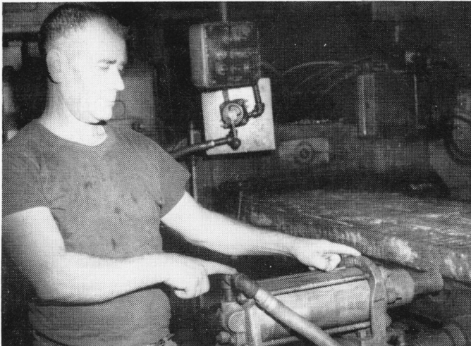
Top left:—Domenico Ianniruberto discovered that merely changing the position of the feed and exhaust lines to the hydraulic aligning cylinder at the Sundstrand Machine would do away with piping damage, caused by cast bars passing into or out of the machine.
